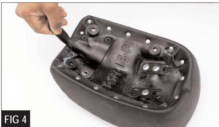
9. To install your pillion seat, slide the two rear tabs on the saddle into the two rear towers on the bike, align the front tab and secure with the stock bolts.
