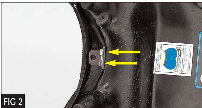
**NOTE:** If the front of the seat is a little loose and has some play, or is a bit too snug, the front tongue can be adjusted as needed by loosening the bolts and moving the bracket up or down (*Figure 2*). The rear bracket is adjustable too and you can add washers under the rear bracket if necessary (*Figure 3*).
