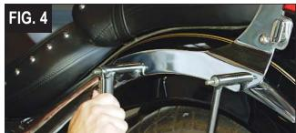
**NOTE:** If not using a sissybar, you need to install an additional 3/16" aluminum spacer onto each stud.
