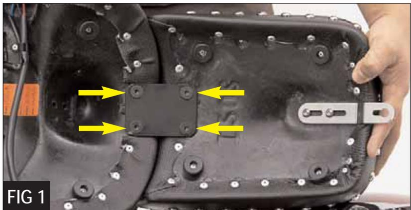
3. If using the pillion pad, bolt the pillion onto the solo seat, using the provided 8mm flat head Allen screws, securing with a 5mm Allen wrench. (Figure 1)
