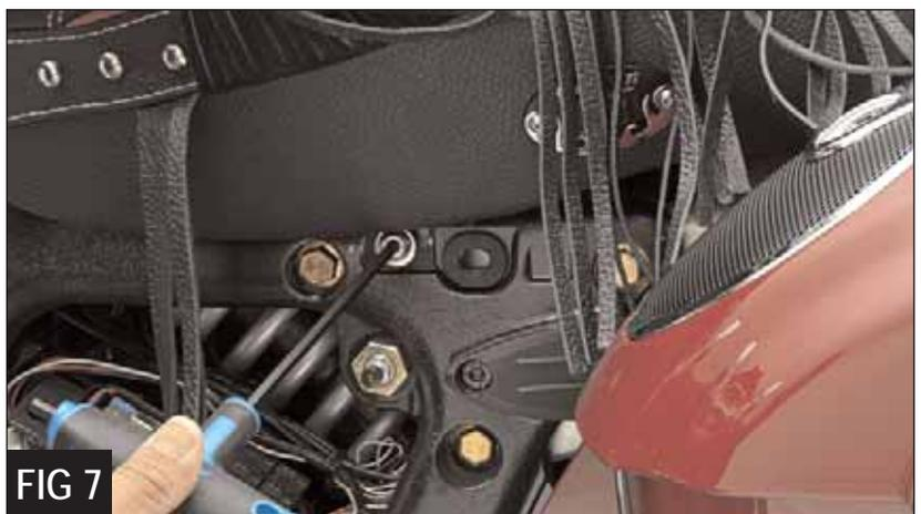
13. Install the solo saddle and luggage rack by sliding the tabs on the solo saddle into place, slowly lower the seat and luggage rack down and secure the luggage rack with the provided 5/16" flat washer and 8mm Allen bolt or stock bolt (Figure 11).
