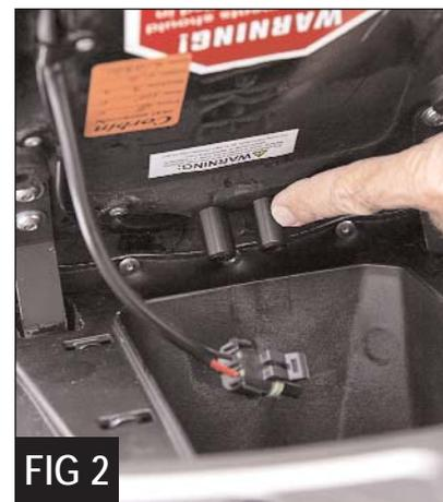
**NOTE:** When mounting the rear seat, the pins shown in *Figure 2*, must clear the front lip of the toolbox while lowering in place.
