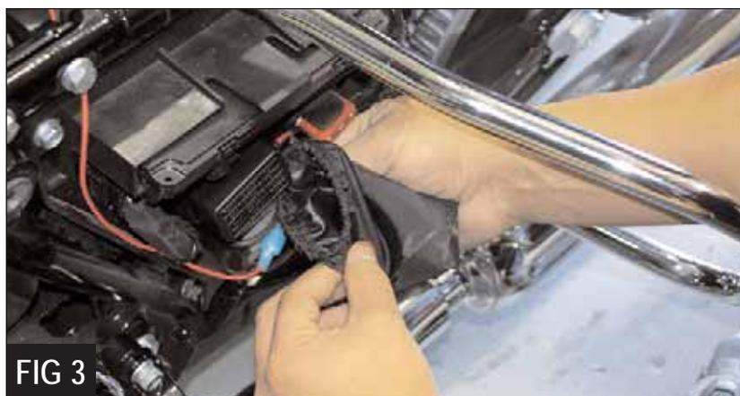
9. Connect the fuse adapter to the wiring harness (Figure 4).
