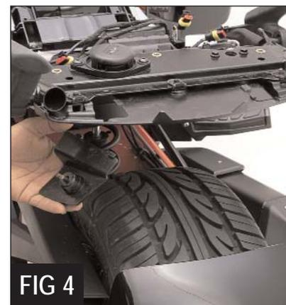
5. Remove the three bolts from underneath the splash guard (*Figure 3*) and gently pull down the taillights (*Figure 4*).
