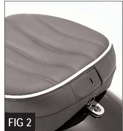
3. Touring Pillion mounts with a tab in the front that sits on top of the Solo Saddle mounting tab and secures with the provided m6 x 25 Allen bolts and flat washers and then securing the rear with the stock bolt (*Figure 2*).
