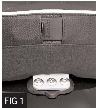
2. To install your Classic Solo saddle, slip the front tab of your saddle under the front seat mount at the rear of the gas tank, then align the rear mounting tab to the subframe and secure with the stock bolts (*Figure 1*).
