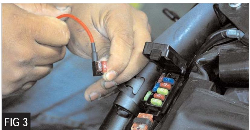
7. Attach the fuse adapter to the red wire on the wiring harness (Figure 7).
