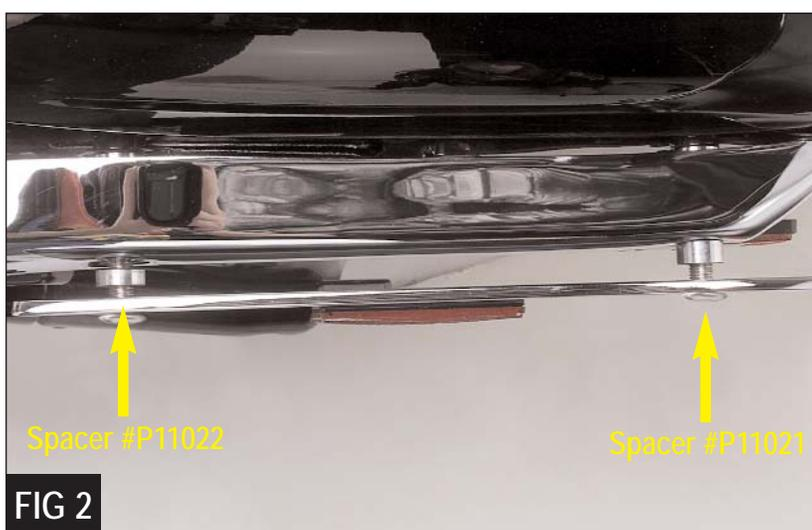
**NOTE:** Use spacer #P11021 (large) in the rear position and spacer #P11022 (small) in the front position or you can use the spacers that came with your sissy bar assembly.
