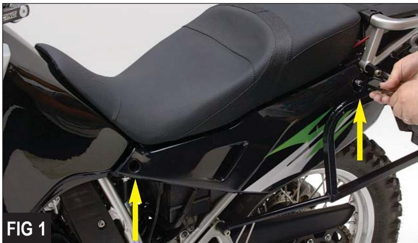
2. Next remove the 6mm hex head bolt on the left and right side of the seat (*Figure 2*), then lift the rear of the saddle up and rearward to remove it.
